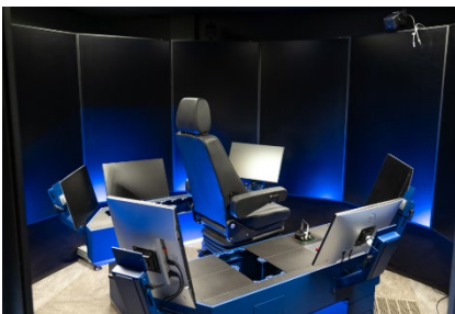
Multi-Purpose Simulator (MPS) with 360 degrees projection for coupled tug or crane simulations.
