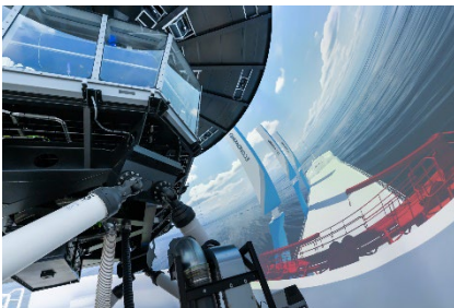
The Large Motion Simulator (LMS) with moving bridge of 4,5 x 5,5 m on a hexapod.
